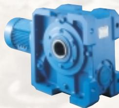
PM Series are helical / worm geared motor units available in six sizes, up to 90kW capacity. A wide range of mounting and shaft options are available. The standard unit has ratios from 8:1 to 307:1 and when combined with RS Series helical gear units, offer ratios of up to 20,000:1.
